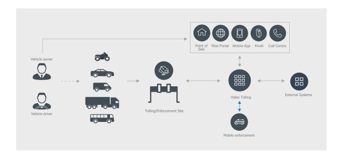
Our Video-based Electronic Toll Collection System is a flexible, state-of-the-art solution for free flow toll collection using video technology. It relies on cameras and computer and AI algorithms to identify and record vehicles passing through designated tolling points. Video Tolling System offers several benefits over traditional tolling methods.
